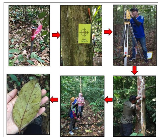
Figure 3: Process involves during field inventory; (a) show the subplot; (b) ID tree tagging; (c) position of tree survey; (d) DBH measurement; (e) Tree height measurement and (f) Tree species identification
